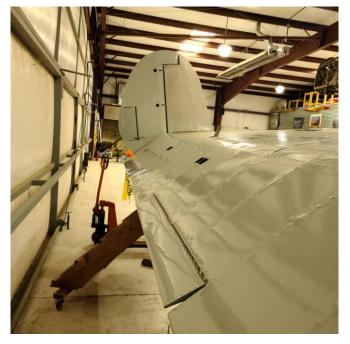
At the aft of the plane the horizontal stabilizers have been finalized, the rudder trim system is in and the elevator trim is near completion. Currently the fairings are being refitted and evaluated for any further action.
