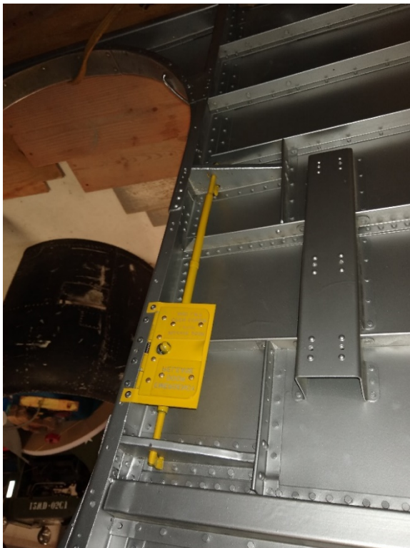
Completely finished Emergency Cabin Door release.
